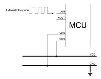
Note: The GND of external oscillator circuit must be as near as possible to VSS pin of micro-controller.
